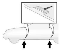
Find the jacking location using the diagram above and corresponding V-shaped locating notches located in the plastic molding.
